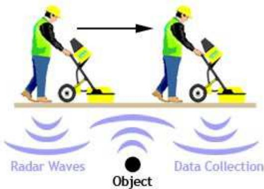
**Figure 3: Working of a GPR.**
