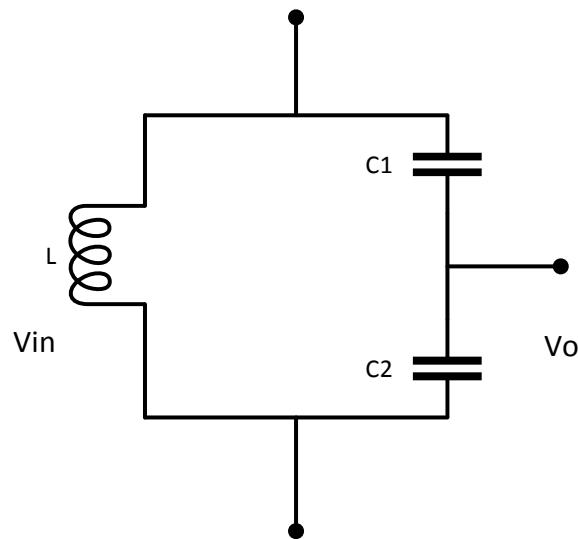
**Figure 4: Capacitance Voltage Divider.**
